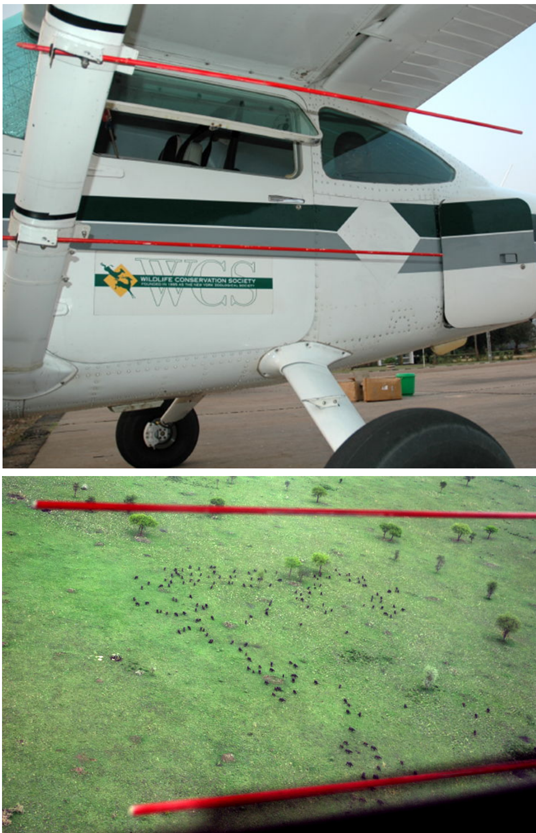
Figure 4: Parallel streamers on Cessna wing strut, and view of strip.
