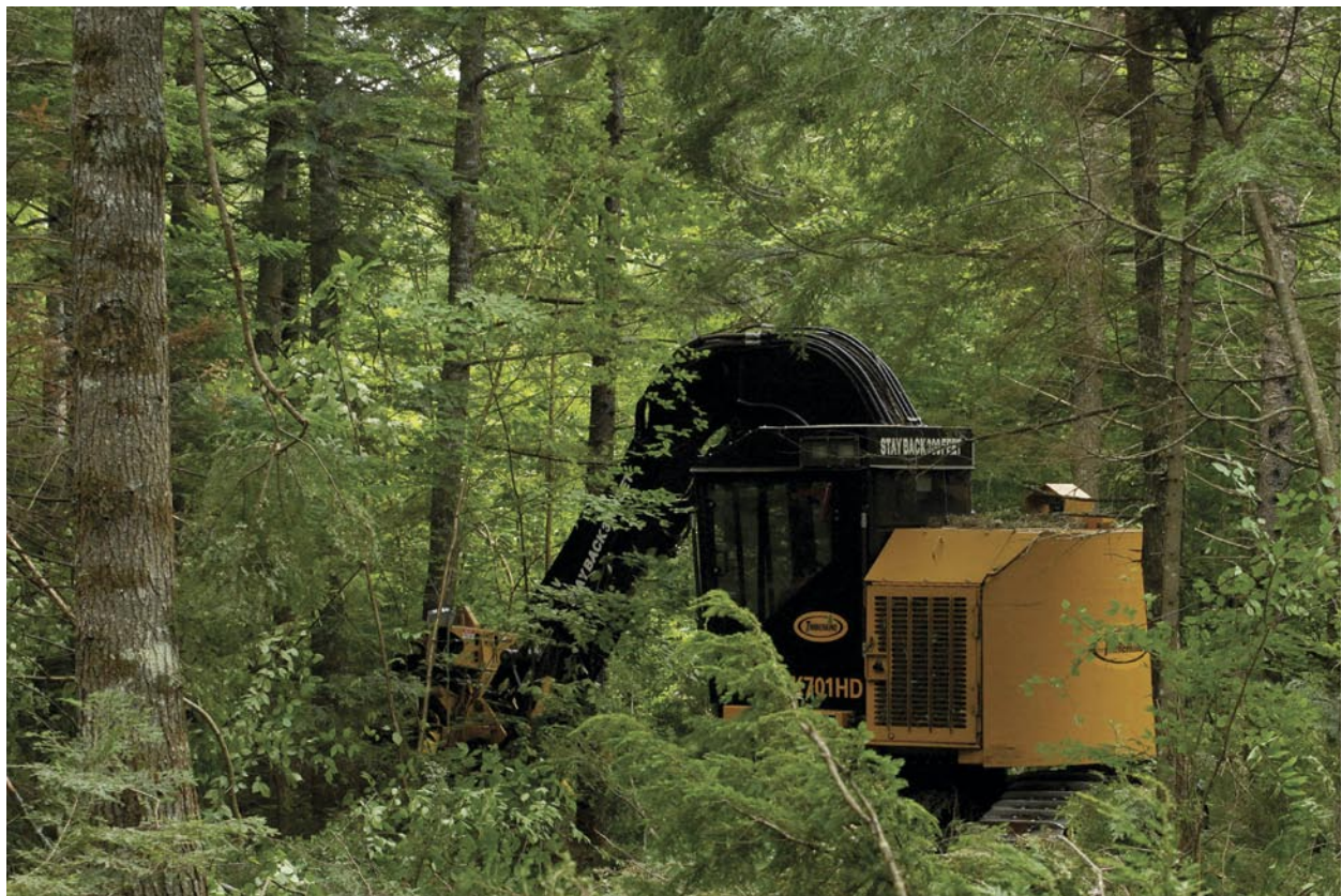
Mechanized cutting: Timberking cut-to-length machine thinning hemlock, Grand Lake Stream, Maine.
