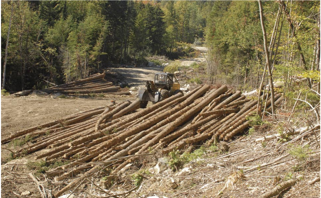
Hand cutting: cable skidder, logs cut and limbed by chainsaw.
